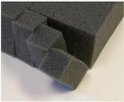
This is probably the easiest and most effective way to seal cable cutouts and floor penetrations. PolarDAM's self-forming foam conforms to any area where it is inserted, blocking cold air from escaping into open spaces. The foam sheets are scored into a "tear-to-size" perforated 1"x1" grid so they can be easily separated along the perforations
